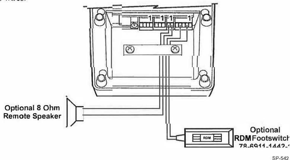
**Figure 8. Connecting Optional Accessories to Station Selector**
