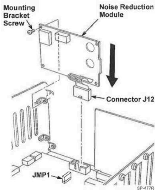
**Figure 3. Noise Reduction Module Installation**
